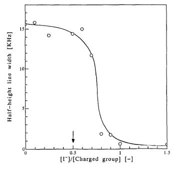
Figure 5 Half-height line width in <sup>79</sup>Br n.m.r. against the molar ratio of I<sup>-</sup> ion to the charged group of poly(BBABr), [I<sup>-</sup>]/[charged group], in various concentrations of NaI solutions at 30°C. The arrow indicates the cloud point of the solution
