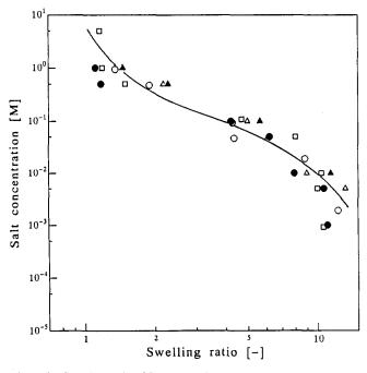
Figure 2 Swelling ratio of BBABr gel in aqueous solutions of various inorganic electrolytes containing different cations: ○, HBr; △, LiBr; □, NaBr; ●, KBr; ▲, NH<sub>4</sub>Br
