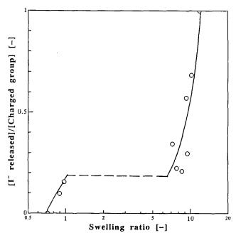
Figure 7 Relation between the molar ratio of I<sup>-</sup> ion released from the BBABr gel to the charged group, [I<sup>-</sup> released]/[charged group], and the swelling ratio of the BBAI gel at 30°C
