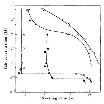
Figure 3 Swelling ratio of BBABr gel in aqueous solutions of various inorganic electrolytes containing different anions: ○, NaCl; △, NaBr; □, NaI; ●, NaClO<sub>4</sub>
