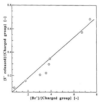
Figure 6 Relation between the molar ratio of  $I^-$  ion released from the BBAI gel to charged group,  $[I^-$  released]/[charged group], and the molar ratio of  $Br^-$  ion in the outer solution to the charged group at  $30^{\circ}C$
